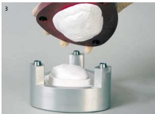
Apply plaster to the model and to the PolyMaster cover, and then close.
