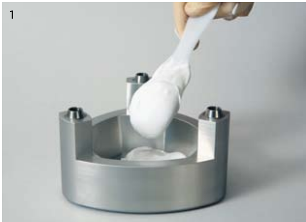
Fill the bottom section with plaster.
